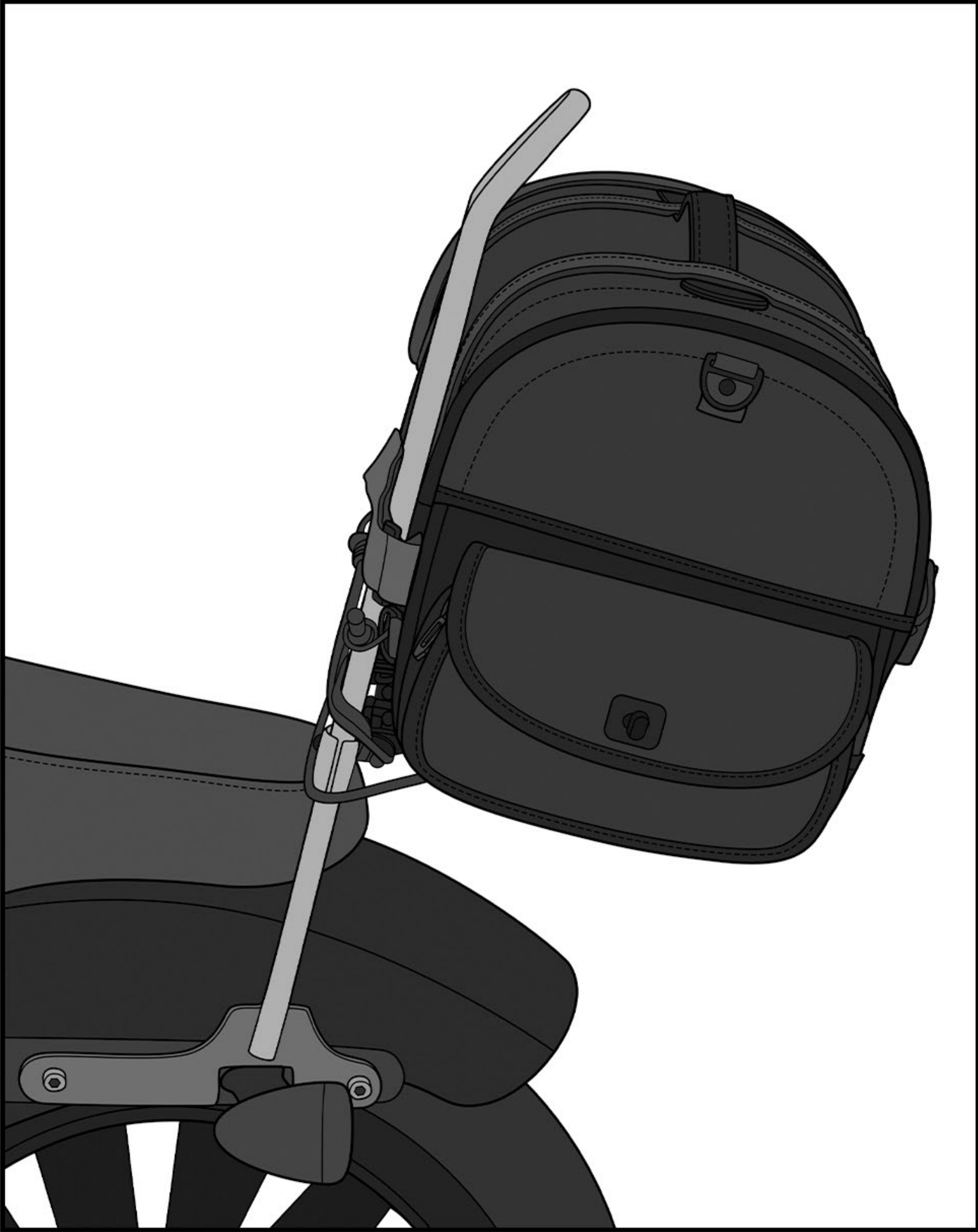
Fig (A) Bag Installed to Sissy Bar
