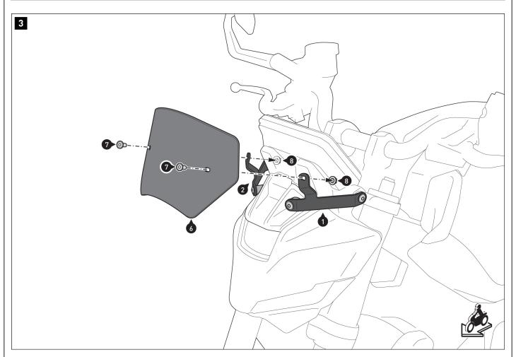
Screw the windscreen (6) to mounting brackets (1) and (2). Tighten the screws as specified.
