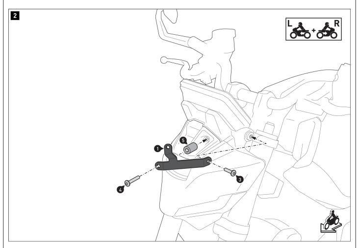
Then screw mounting brackets (1) and (2) onto the vehicle.
