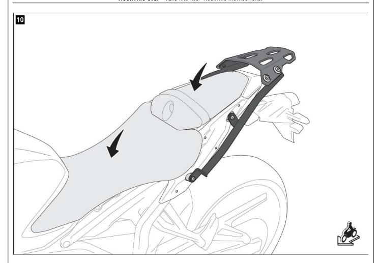
Reattach the seat and passenger seat to the vehicle.
