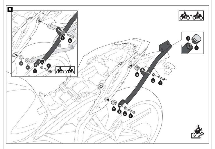
⚠ NOTE: If the SW-MOTECH side carrier is mounted at the same time, the attachment parts (7) and (8) are omitted. Instead of these attachments, mount the side support(s) using the attached attachments (\*) as shown in the detailed drawing.
