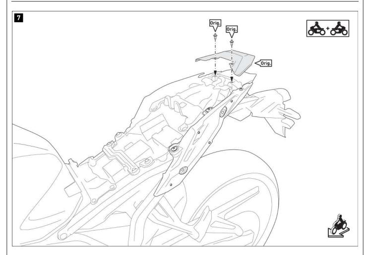
Mount the rear panel on the vehicle using the original plastic dowels.
