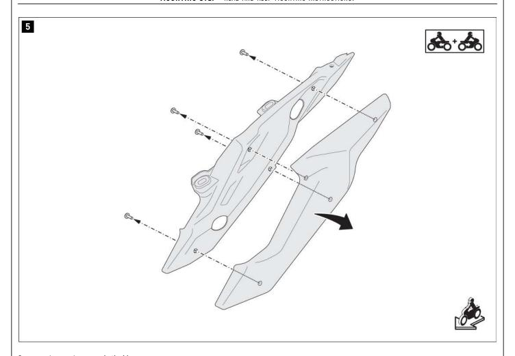
Separate the panel parts on **both sides**. The outer cladding parts are omitted.
