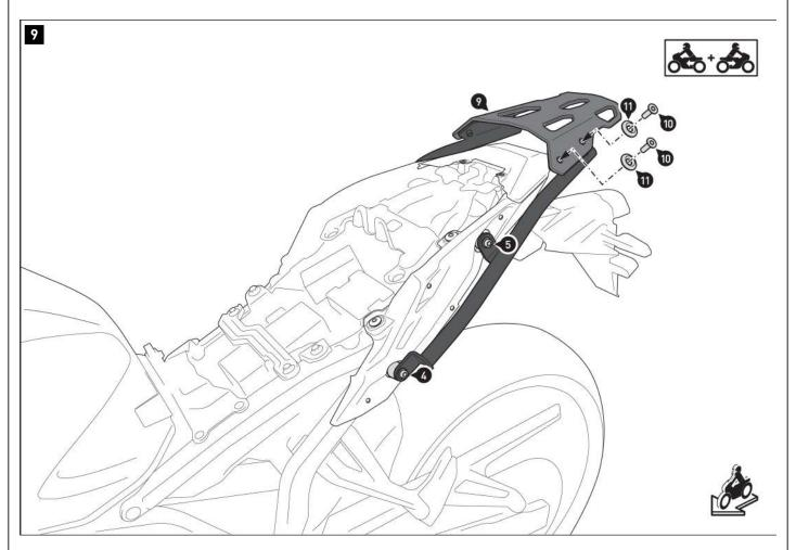
Screw the rack [9] onto the mounting struts (1) and (2). **A WARNING:** Use a liquid threadlocker!
