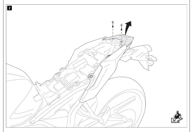
Loosen the two plastic dowels, and remove the rear panel from the vehicle.
