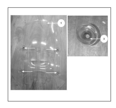
**2** Loosely assemble the screen mount clamp (4) with an M5 bolt (12) and nut (14). Repeat this step with remaining 3 No. mount clamps.
