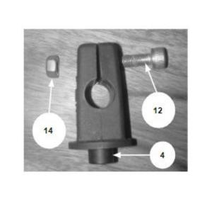
**3** Push fit an M5 nut (14) into the pocket of the 4 No. screen mount clamps (4) and loosely assemble to the touring screen (1) through the rubber grommets (3) with an M5 bolt (10) and M5 washer (16).
