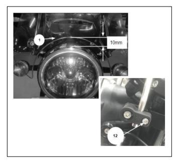
**12** Tighten 4 No. M5 bolts (11) to *3Nm*.
