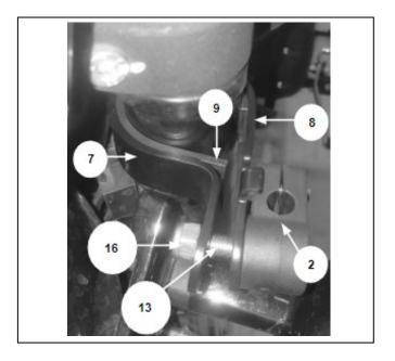
**9** Align the fork clamp assembly so that it butts up to the top surface of the fork tube. Using the trafficator mount bracket as a guide, position the clamps parallel to the bracket and tighten the M8 nyloc nut to **25Nm**. Repeat this step for the other fork assembly.
