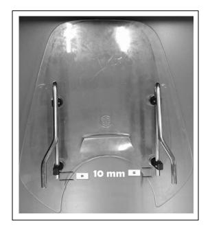
**7** Loosely assemble the lower mount (2) with an M6 bolt (12) and M6 nut (15). Repeat this step for the remaining lower mount.
