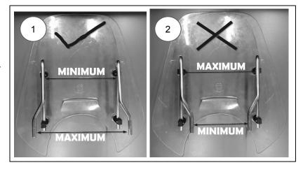
**6** Ensure equal distance of 10mm is maintained on both sides of the mount rods as shown in the image.
