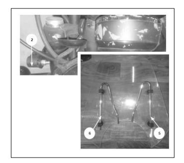
**11** Position the touring screen (1) at the desired height. A minimum 10mm gap between the headlight bezel is recommended. Ensure that the screen is central to the bike then tighten 2 No. M6 bolts (12) to **4Nm**.
