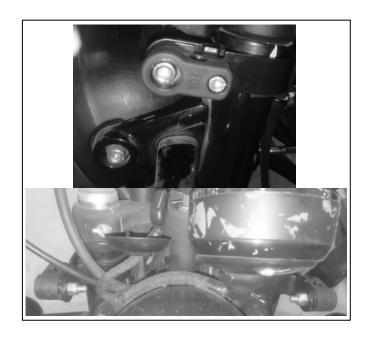
10 Slide the touring screen mount bars (5,6) into the lower mounts (2).
