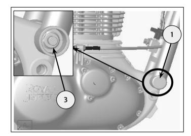
**6** Insert Engine guard, Right Hand (1) to the vehicle cradle assembly (2) approximately position as shown.
