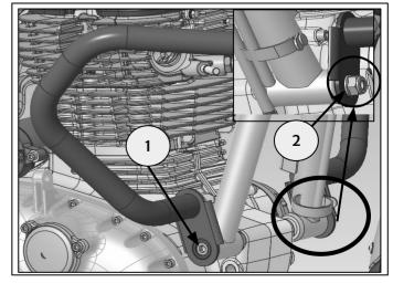
**9** Position engine guard assembly top side with vehicle cradle assembly as shown. Use fixings (1) and nuts (2) from the kit and tighten to **25Nm**.
