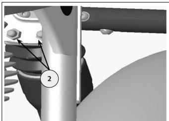
**10** Tighten engine guard bottom mount fixing (1) and nut (2) to *55Nm*.
