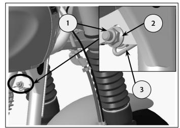
**4** From step 1 use Top mount assembly (2) and from kit use engine guard assembly, Left Hand (1). From kit use M6 x 16mm fixings (3) and washers (4) to clamp Top mount assembly (2) to engine guard assembly, Left Hand (1) as shown. Tighten to **8Nm**.
