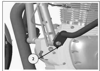
**11** Position Exhaust pipe assembly to Engine head and silencer assembly as shown, Reuse the fixings (2),(3), and nut(4) retained in step 2. Connect the O2 sensor cable (1) to vehicle.
