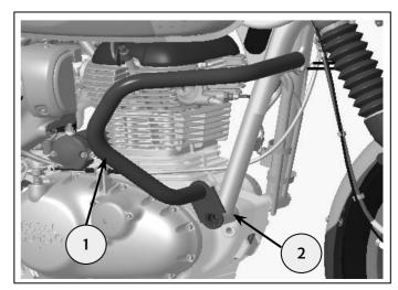
**7** Insert pre assembled Engine guard, Left Hand assembly (2) from step 4 with the vehicle cradle assembly (3) and Engine guard, Right hand (1). Rotate and position to accommodate insertion of washers(4) and M6 x 16mm fixings (5) from kit, as shown. Tighten fixings to 8Nm
