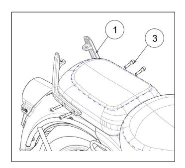
**4** Assemble the Backrest pad (2) with 2 quantities of Bolt, cap, M8 x 40 (3). Tighten the bolts to **25Nm**.
