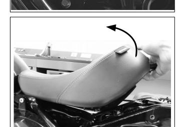
**3** Push the front of the new accessory rider's seat on to the fuel tank tab and locate steel inserts into rubber mounts on the supporting bracket.
