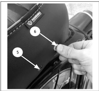
**7** Remove passenger seat by lifting at the rear and pulling rearward.
