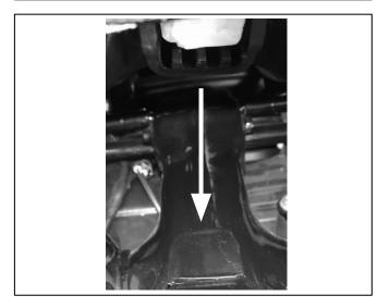
**4** Insert the 2x Hex Flange Head Bolts (1) and washers (2) that were removed in step 1 into seat base threaded inserts. Torque to **10NM**.
