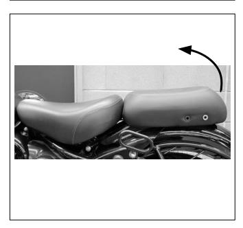
**8** Re-fit short (5) and long (6) inserts into new accessory seat as shown. Inserts locate into grommets. Repeat on other side.
