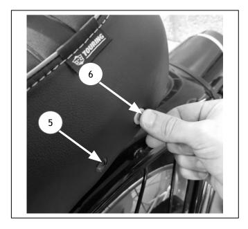
**9** Fit new accessory passenger seat by locating front hooks into features as shown and then lowering down to align inserts (5 and 6) with threaded holes in subframe.
