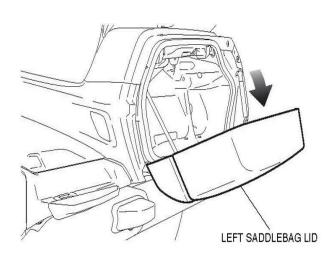
2. Remove the left side cover as shown. Disconnect the Negative (-) cable from the battery.
