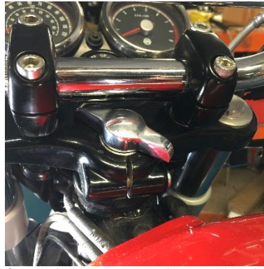
26. Adjust steering damper knob to your desired resistance.
