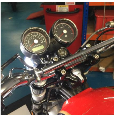
24. Lift handlebars back into position.
