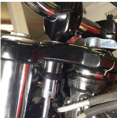
25. Refit riser bolts under top yoke. Torque: 45 N-m.
