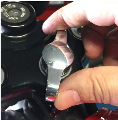
23. Tighten steering damper knob until it bites.
