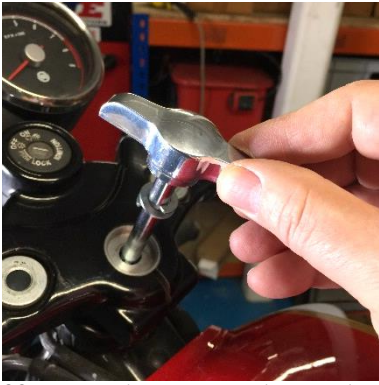
22. Insert the steering damper knob with spring washer on the rod and insert into modified steering damper stem nut.
