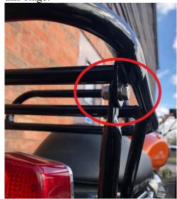
5. At this stage now check all the fixings are secure. If you are fitting our side pannier frames (92848A) in addition to this large rack, you will need to utilise the additional brackets and fixings as shown below.
