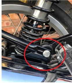
4. Then, mount the top of the support bar to the inside fixing on the rack using the shorter M6 bolts supplied, as shown below. it may be necessary for a "tweak" of the support bar to line up at this stage.
