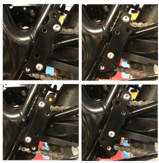
2. There are four recommended positions on the adjustment plate by using the two different untapped mounting holes and turning the plate over. (There are other positions but care must be taken if using these that the brake and gear lever have full travel and that any associated fittings/pipes are not stressed and cannot be trapped).
