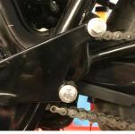
Undo the gear change linkage (10mm nut) and remove the connection from foot gear change lever. Undo foot peg hanger 12mm bolts and remove foot peg hanger.
