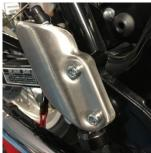
Remove split pin and fulcrum pin from brake lever/brake cylinder joint. Loosen M6 cap head screws and remove brake cylinder guard.
