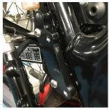
Carefully move the brake master cylinder to access the foot peg hanger. Remove the M8 flanged bolts and remove the foot peg hanger. Synchronise the position of the mounting holes on the adjustment plate with the gear change side. Attach the adjustment plate to the frame using the M8 x 30mm button head screws, (depending on the position you
