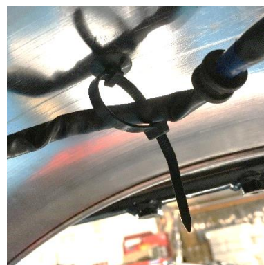
20. Pull the excess wiring back through towards the panel area. Use the heat shrink, cable ties and wiring holders, ensuring a tight fit along the underside of mudguard.
