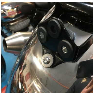
10. Use the M6 button head screw through the frame hole and the mudguard with the flat washers/nyloc, then tighten the button head screw and the two bolts.
