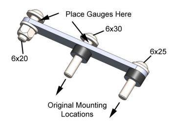
4. Bolt the riser clamps to the adapter plate using the included flat head bolts. **IMPORTANT:** These bolts must have the threads completely coated with blue threadlocking compound before installation.
